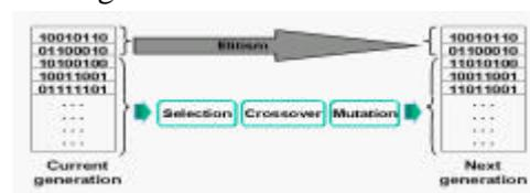
Figure 3. Producing the next generation in GAs.
